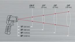
This meter is configured with a 20:1 optical resolution (distance-to-spot ratio). The distance-to-spot ratio defines the size of the measurement area relative to the distance between the measurement location and the IR sensor.
