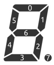
Note that even though we call these *seven*-segment displays there are actually 8 LEDs in each one because of the decimal point.
