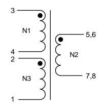
Application of transformer allows for leadwires between terminals 7&8 to solder bridge.
