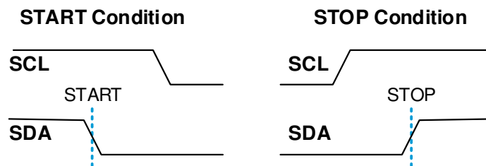
Figure 5. START and STOP Condition Waveform
