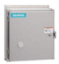
Mechanically held lighting contactor, Contactor amp rating 30Amp 0NC  $\_$  4NO poles, 208VAC 60HZ coil, Non-combination type, Encl NEMA type 4X 304 S-steel Water/dust tight noncorrosive
