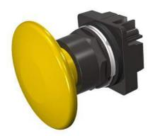
30mm BlackMax, Epoxy Coated Corrosion Resistant Metal Operator, Round Push-Pull Operator Non-Illuminated Mushroom Head Cap Large 2 1/2" (63.5 mm) Plastic, Yellow 2 Position Maintained, Pull-to-Release UL Listed, CSA Certified NEMA 1,3,3R,4,4X,12,13 & Automotive Standards
