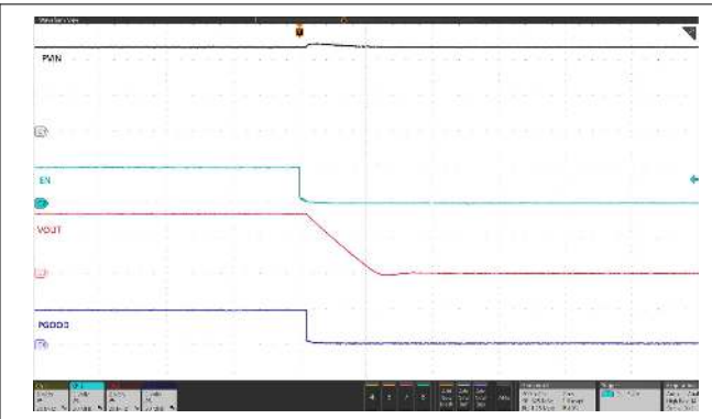
Figure 7-18. VOUT_B Shutdown From Control, 25-A CC Load
