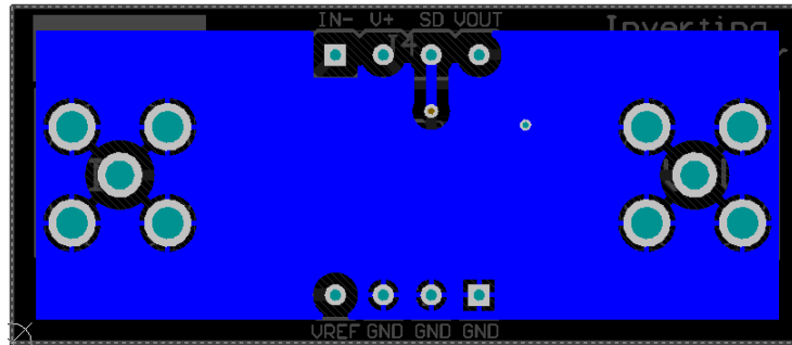
Figure 32. Inverting Comparator Bottom Layer
