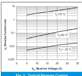
. 1. Typical Forward Voltage Fig. 2. Typical Reverse Current
