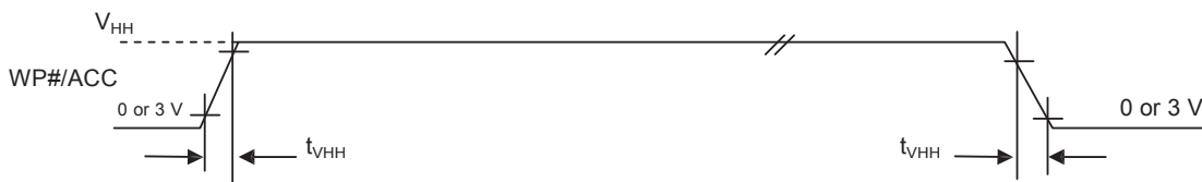
Figure 11. Accelerated Program Timing Diagram
