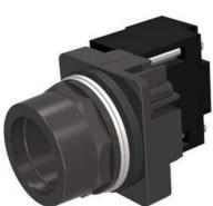
30mm BlackMax, Epoxy Coated Corrosion Resistant Complete Metal Unit Illuminated Push-Pull Operator Transformer type, 240V AC Incandescent Lamp Less Mushroom Head Cap 3 Position Pull-Momentary/Push-Maintained UL Listed, CSA Certified NEMA 1,3,3R,4,4X,12,13 & Automotive Standards
