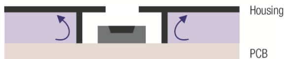
Figure 2: Sealing of the sensor compartment towards the remaining housing minimizes the influence of entrapped air on the sensor.
