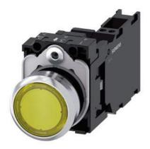
Illuminated pushbutton, 22 mm, round, metal, shiny, yellow, pushbutton, flat, momentary contact type, with holder, 1 NO+1 NC, LED module with integrated LED 24 V AC/DC, Spring-type terminal
