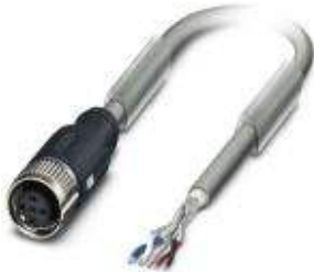
Bus system cable, CANopen®, 5-position, PUR halogen-free, Gray RAL 7001, Free cable end, on Socket straight M12-SPEEDCON, A-coded, Cable length: 15 m
