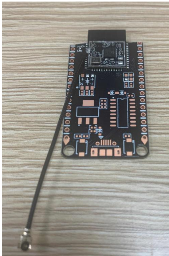
Figure 8 Schematic diagram of the antenna test prototype
