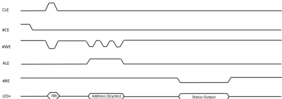
Figure 9-8 Read Status Enhanced (78h) Operation
