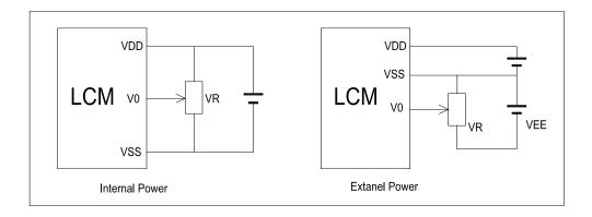
V<sub>DD~</sub>V<sub>0</sub>: LCD Driving voltage VR: 10k~20k
