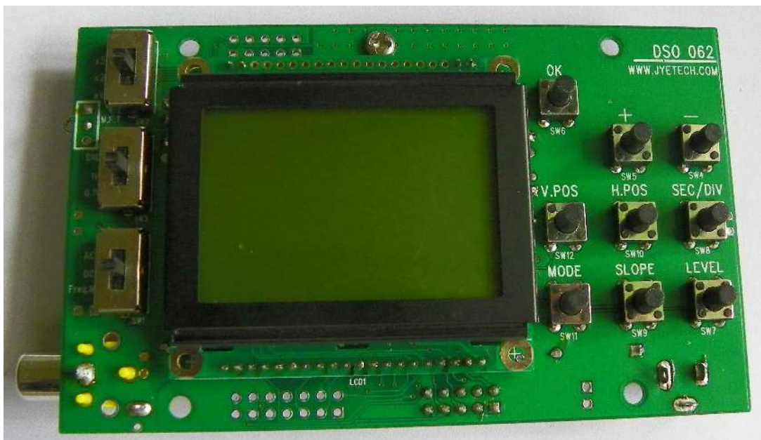
All on-board components soldered (front side)
