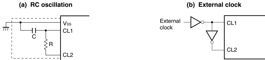
Figure 5-10. External Circuit of External RC Oscillator
