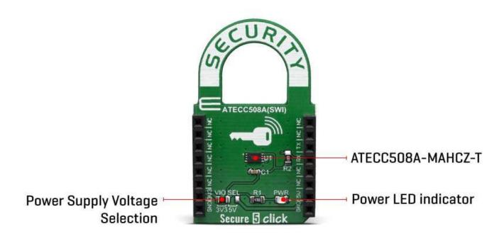
It features a wide array of defense mechanisms specifically designed to prevent physical attacks on the device itself, or logical attacks on the data transmitted between the device and the system. Hardware restrictions on the ways in which keys are used or generated provide further defense against certain styles of attack.
