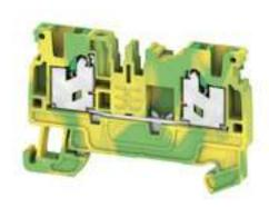
A protective feed through terminal block is an electrical conductor for the purpose of safety and is used in many applications. To establish the electrical and mechanical connection between copper conductors and the mounting support plate, PE terminal blocks are used. They have one or more contact points for connection with and/or bifurcation of protective earth conductors.
