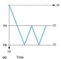
(x) Time (y) Vacuum (1) Adjustable value PH: High point PB: Below point
