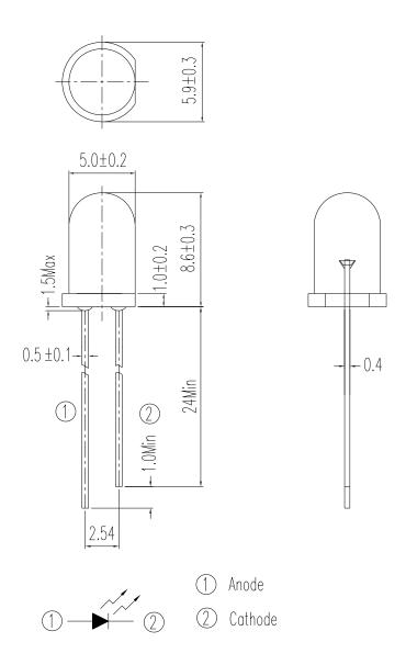
Note: Tolerances unless dimensions ±0.25mm
