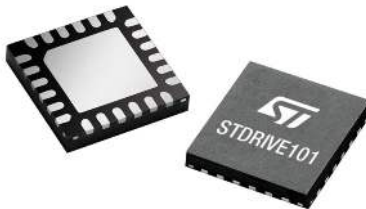
VFQFPN 4 x 4 x 1.0 mm 24 leads pitch 0.5 mm
