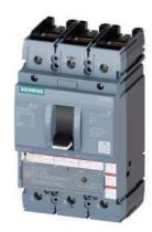
circuit breaker 3VA5 UL frame 250 breaking capacity class H 65kA @ 480 V 3-pole, line protection TM230, FTAM, In=90A overload protection Ir=90A fixed short-circuit protection Ii=5...10 x In cable connection on both sides
