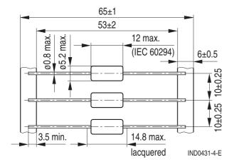
Dimensions in mm Minimum lead spacing 15 mm
