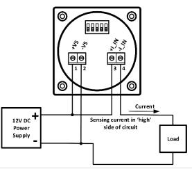
It is also possible to use the meter to monitor voltage in a circuit that is independent of the meter's power supply circuit, as shown in the schematic below. When used in this way, the meter's current measuring terminals may electrically float with respect to its power supply terminals, as long as the voltage difference between the two terminal pairs remains within +/- 48V of each other.
