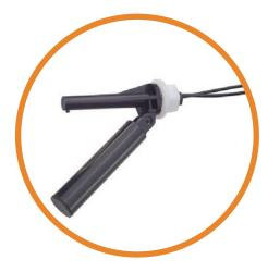
The RSF30 is a higher power side entry, internally fitted switch. These may be used for directly switching some small loads of less than 100VA. Fitting of this type requires access to the inside of the tank.
