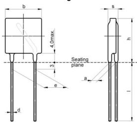
16.5  $b_{max}$  $h_{\text{max}}$ 19.5 S<sub>max</sub> 8.6 = 10.0 ±1.0 е 4.6 ±1.0 а  $I_{min}$ = 25.0 = 1.0 ±0.05  $\emptyset d$
