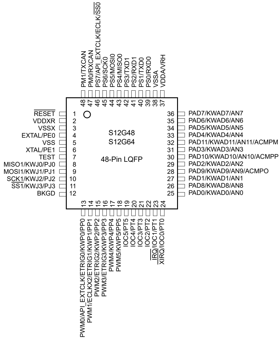
Figure 1-11. 48-Pin LQFP Pinout for S12G48 and S12G64
