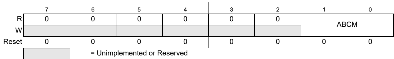
Figure 8-6. Debug Control Register2 (DBGC2)
