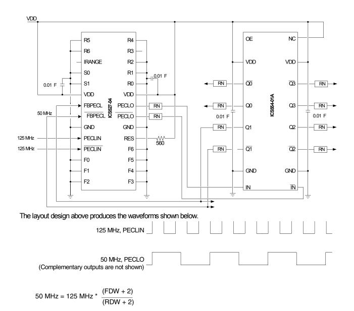
FBPECL pair pins are connected to the Q1 outputs (chosen arbitrarily) of the ICS554. This aligns all the outputs of the ICS554 with the 125 MHz input since the ICS527-04 aligns rising edges on the PECLIN and FBPECL pins.
