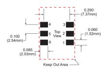
Keep Out Area Note: Do not route any traces under the device in the keep out area.
