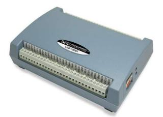
USB-1808 Series devices provide eight simultaneously-sampling analog inputs that are configurable per channel as differential or single-ended, two analog outputs, four digital I/O, two general-purpose counters, two quadrature encoders, and two timer outputs.
