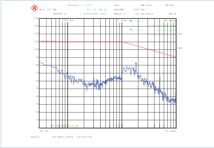
Figure 11 — Peak scan for the BLACK lead with C_{IN-1} = 100\mu F , C_{OUT} = 2000\mu F , 100% load
