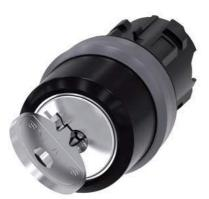
RONIS key-operated switch, 22 mm, round, plastic with metal front ring, lock number 455, with 2 keys, 2 switch positions O<I, momentary contact type, Actuating angle 45°, 10:30h/12h, key removal O, with laser labeling, inscription or symbol Customer-specific selection with SIRIUS ACT configurator (CIN)
