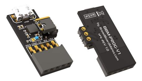
The BBM-PROG features a 3-pin jumper with shunt, which is present to change the way the programmer handles the Reset line, utilised by TED-96 and other devices.
