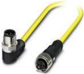
Sensor/Actuator cable, 4-position, TPE, yellow RAL 1021, Plug angled M12 SPEEDCON, A-coded, on Socket straight M12 SPEEDCON, A-coded, Cable length: 3 m
