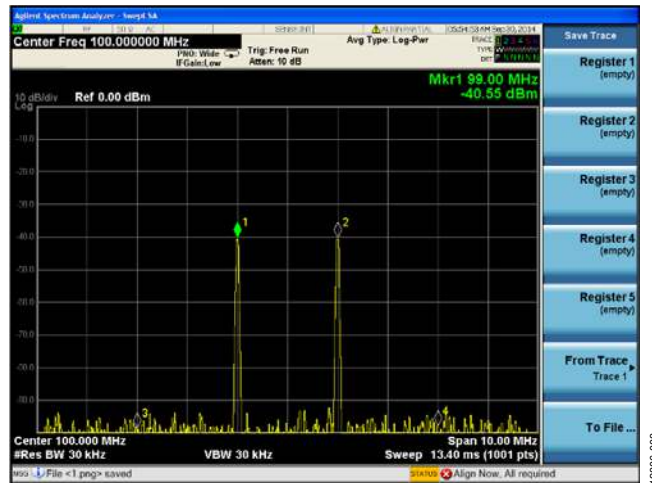
Figure 8. Spectrum Analyzer Screen, CW Generators Set for -40 dBm/Tone on ADA4961 Output
