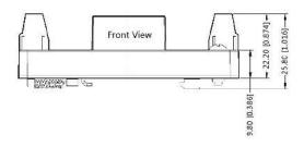
Note: Unit: mm[inch] Mounting rail: TS35 Wire range: 24-12 AWG
