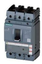
circuit breaker 3VA5 UL frame 250 3-pole, starter protection TM120M, AM, In=200A without overload protection short-circuit protection Ii=6...12 x In nut keeper kit on both sides
