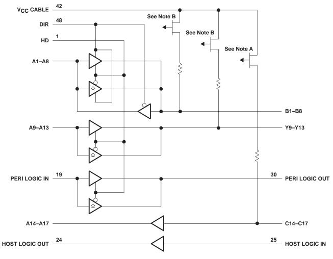
NOTES: A. The PMOS transistor prevents backdriving current from the signal pins to V<sub>CC</sub> CABLE when V<sub>CC</sub> CABLE is open or at GND.
