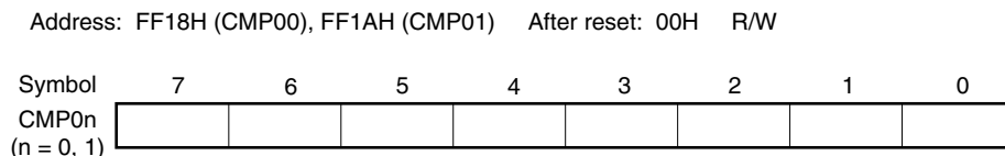
Figure 8-3. Format of 8-Bit Timer H Compare Register 0n (CMP0n)
