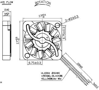
Sunon standard sample exclude the connector. If there is any request for connector, please advise in advance. About recommend connector, SUNON recommend the following models for SUNON Mighty Mini Fan/Blower: 1.(JST) SUR series connector: 02SUR-32S / 03SUR-32S.
