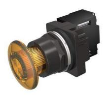
30mm BlackMax, Epoxy Coated Corrosion Resistant Complete Metal Unit Illuminated Push-Pull Operator Transformer type, 240V AC LED Lamp Mushroom Head Cap Small 1 3/4" (44.5 mm) Plastic, Amber 3 Position Pull-Momentary/Push-Maintained UL Listed, CSA Certified NEMA 1,3,3R,4,4X,12,13 & Automotive Standards
