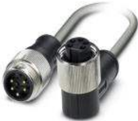
Bus system cable, DeviceNet, 5-position, PUR halogen-free, Gray RAL 7001, Plug straight 7/8"-16UNF, on Socket angled 7/8"-16UNF, Cable length: 0.5 m
