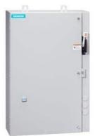
Non-reversing motor starter Size 3 Three phase full voltage Solid-state overload relay OLRelay amp range 25-100A 190-220/220-240V 50/60HZ coil Combination type 100A fusible disconnect 100A/250V fuse clip Enclosure NEMA type 4/12 Water/dust tight weather proof Standard width enclosure
