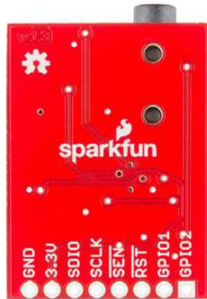
Underside of breakout board showing pin labels
