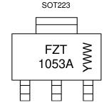
FZT1053A = Product Type Marking Code YWW = Date Code Marking Y or  $\overline{Y}$  = Last Digit of Year (ex: 9 = 2019) WW or  $\overline{W}W$  = Week Code (01 to 53)
