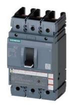
circuit breaker 3VA5 UL frame 250 breaking capacity class H 65kA @ 480V 3-pole, line protection TM230, FTAM, In=225A overload protection Ir=225A fixed short-circuit protection Ii=5...10 x In UL 489 SB (naval), 50 °C without connection
