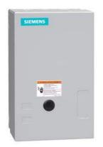
Non-reversing contactor, Size 2 1/2, Three phase full voltage, Contactor amp rating 60A, 3 wire (NO aux included), 24VAC 50-60Hz coil, Non-combination type, Enclosure NEMA type 1, Indoor general purpose use, Standard width enclosure
